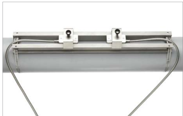
Metallic mounting rail with transducers
