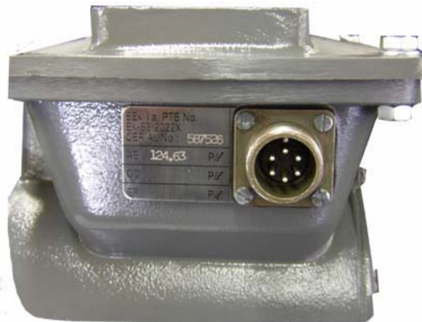
Figure 3 Dataplate with pulse frequency information
