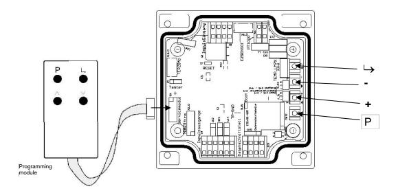
Programming with the programming module is to be performed in the same way as with the buttons..The external and internal buttons correspond to each other in the following way:
