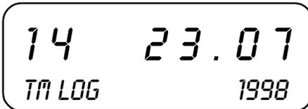
Time and date of the last logged entry. Pressing the RESET key will display the previous logged entries.
