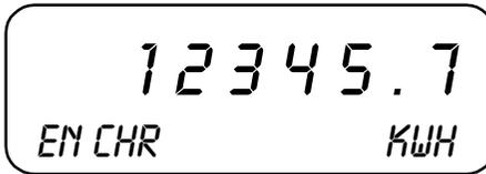
Charge Energy default display - Charge Energy measured since the last reset.
