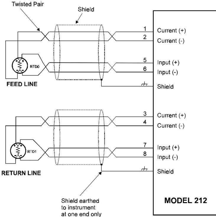
*Note: Care must be taken to ensure the (+) of the current terminal is connected to the same side of the RTD as the (+) of the input terminal. The RTD, itself, has no polarity.*
