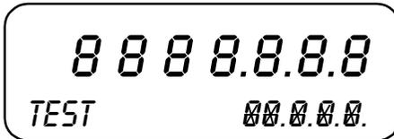
Display segments test. Segments are flashing.
