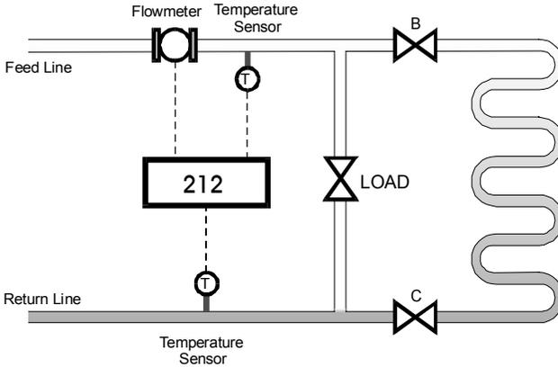
To compensate for any offset in the temperature sensors the Model 212 must be put into the Set-up Program mode. The bypass valve "A" is then opened and the valves "B" and "C" are closed.
