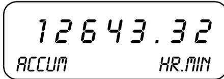
Accumulated operating time (non-resettable).
