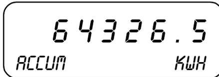
Accumulated Discharge Energy (non-resettable).
