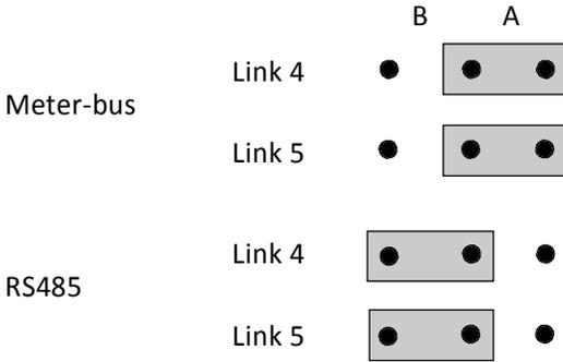
These links are accessible by removing the front panel as detailed in section 7.2 and the link positions are as shown in the drawing in section 7.3. Links are made via small black caps which fit over the connecting posts, thereby creating a link.
