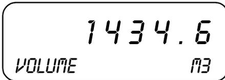
Volume of water measured through the system since the last reset.
