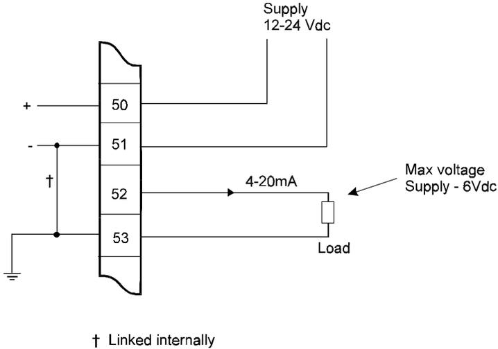
The maximum output voltage is the supply voltage less 6 volts. Therefore the maximum load resistance can be calculated as:
