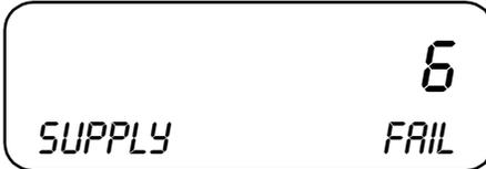
Number of times the power has failed or has been switched off to the unit since the last reset.
