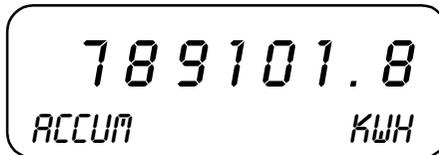
Accumulated Charge Energy Total (non-resettable).
