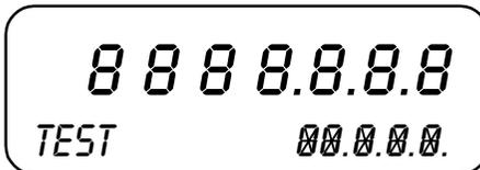
Display segments test. Segments are flashing.
